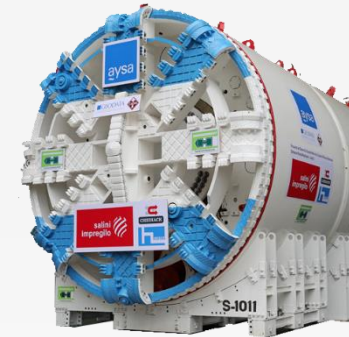
TBM EPB ø4,30m Up To 6 bar
